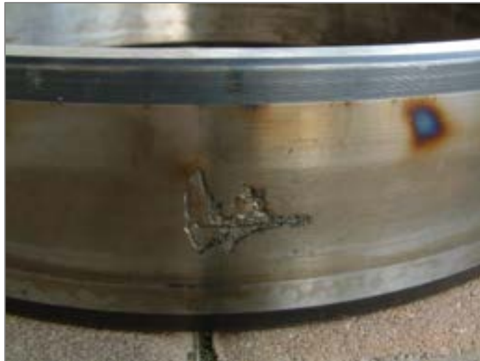
Inner race defect on the flywheel
